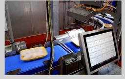
Utilising InVISION Camera Grading System from Foodmate, the system can recognise and sort products according to customer requirements.
